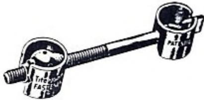
triangle. Insert the draw bolt, now locked in place into the small hole. When it engages the nut begin rotating the nut with an awl or ice pick. This will draw the two pieces of the frame together. Tighten until contact is made and the frame side can still shift easily.
