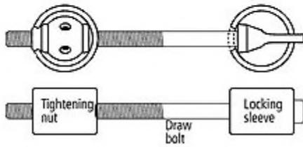
Use the two remaining pieces and repeat the process in the opposite corner. Now put the draw bolts, locking sleeves and tightening nut in the two remaining corners and pull them together evenly. Align each joint and tighten the nut firmly. Screw in corner brackets if provided.
