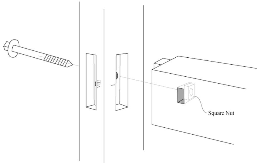
**Note: Loosen the screw holding the bed bolt cover before swinging it out of the way.**
